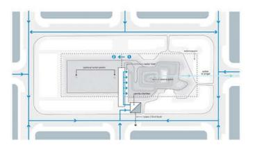
The watersquare requires a clean sewerage system of rainwater only, separate from black and grey water. The principle of water chambers and watersquares is described in the illustrations above.
